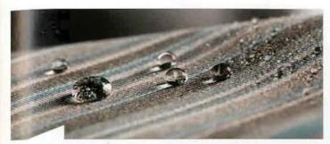
The special surface treatment allows the rainwater draining off to be used for picking up the dirt from the surface of the awning, thereby ensuring a better appearance and longer service live of the awning sheet.
