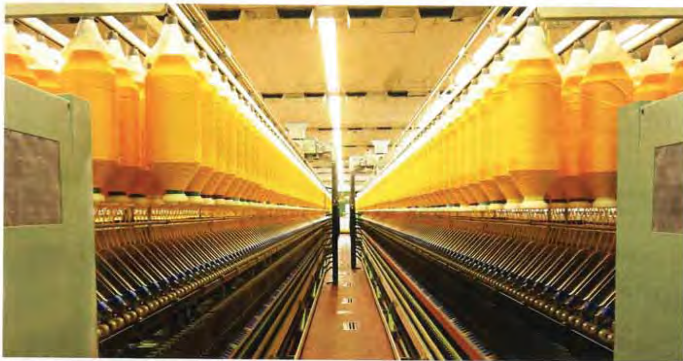
Solution-dyed acrylic yarn being spun at the Lenna, Italy, plant.
