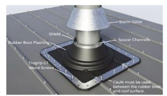
Rubber Boot Flashing: The only certified ventilated Rubber Boot Flashing in the industry! The Rubber Boot Flashing eliminates the traditional need to hammer, bend, and push deadsoft aluminum flashing into shape on a metal roof, saving time and effort. Designed to fit 4'' and 5'' diameter direct vents, 5''-8'' chimneys, and roof pitches up to 12/12 (10/12 for 8'' diameter chimney). Available now! Contact: (800) 835-4429 or www.duravent.com.
